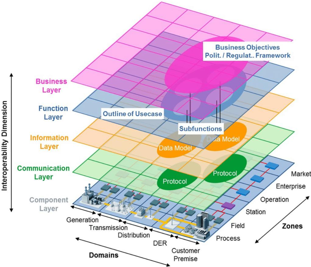
Figure 3: SGAM (Smart Grid Architecture Model)
