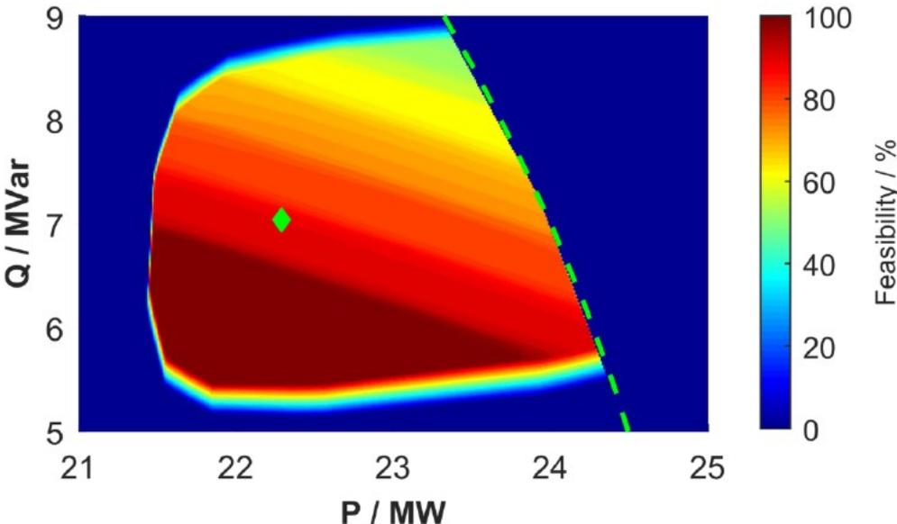
Figure 6: Topology and tap position based FOR feasibility [14]
